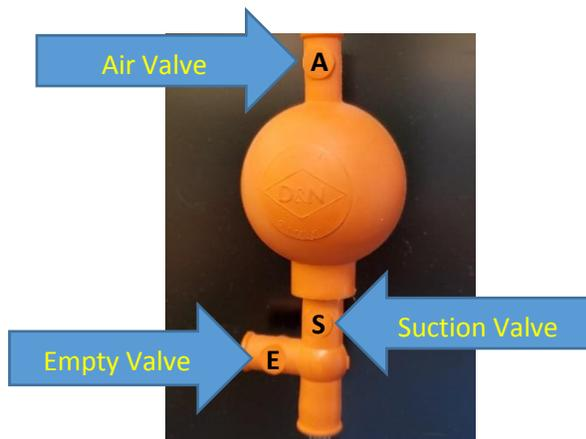
Figure 2. Three-Way-Valve Pipette Bulb
