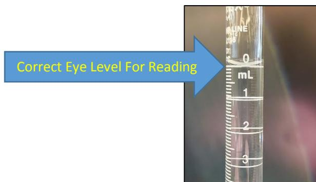
**Figure 7. Initial Volume: 0.00-mL Reading**
